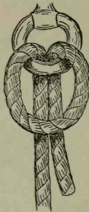
FIG. 31.—Lark's head with toggle (A) withdrawn.
